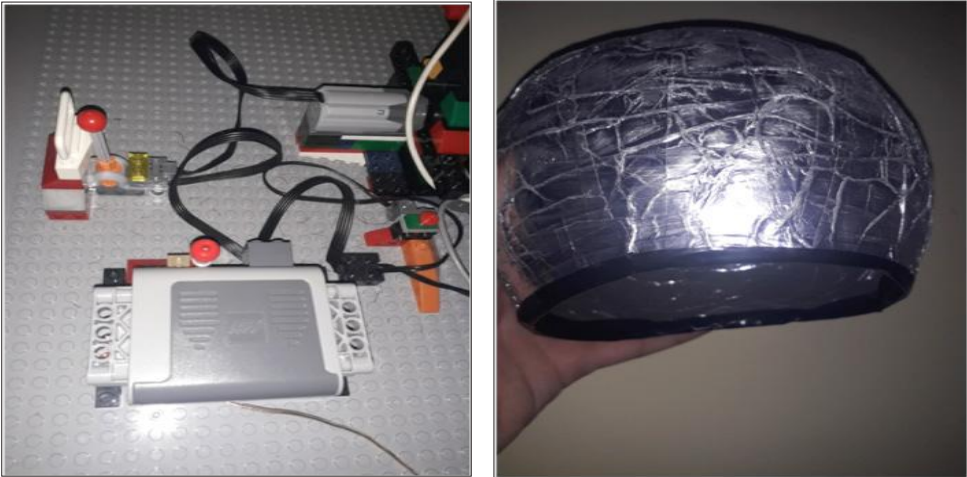
Fig. 2. This is the battery box (6 batteries, each 1.5V, so 9V total ), the controller and the DC motor
