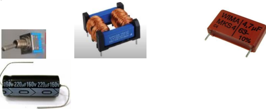
Figure 2. Switch, coil with inductivity 200 mH and condensers with capacity 4,7 \mu F and 220 \mu F.
