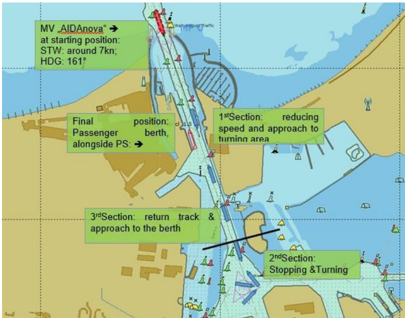
Figure 6. Sample for conventional briefing for a berthing scenario in the Port of Rostock
