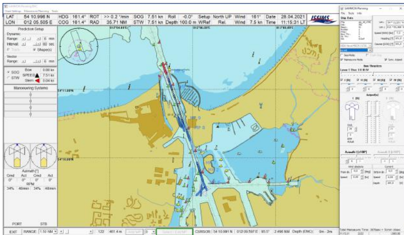
Figure 7. Sample with SAMMON Planning tool for arrival planning for Rostock port: Using new POD strategy with IN-OUT configuration, e.g. speed changes by turning PODs inward
