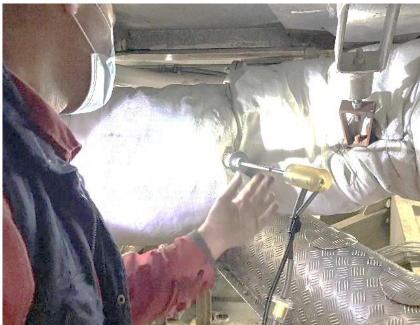
Figure 5. Installation of exhaust sampling probe
