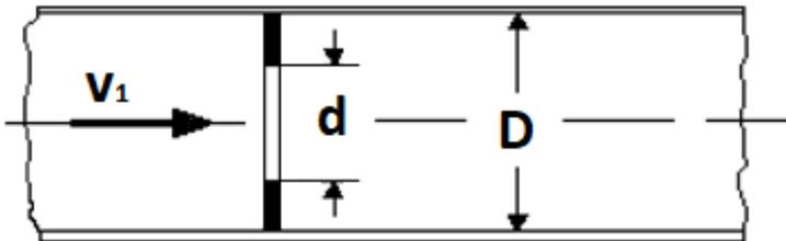
Figure 5. Orifice flow resistance
