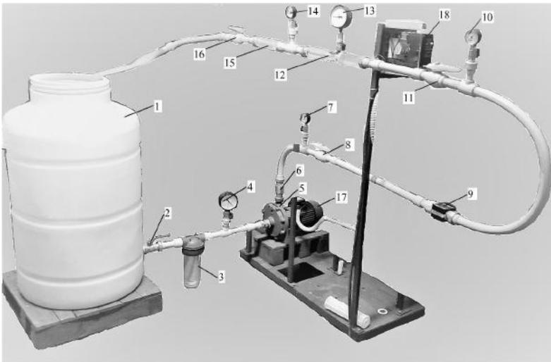
**Figure 1.** Pictorial diagram of the Experimental unit
