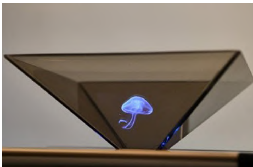
Fig. 6. Volumetric holographic display – inverted reflection pyramid with an underlying tablet as image source
