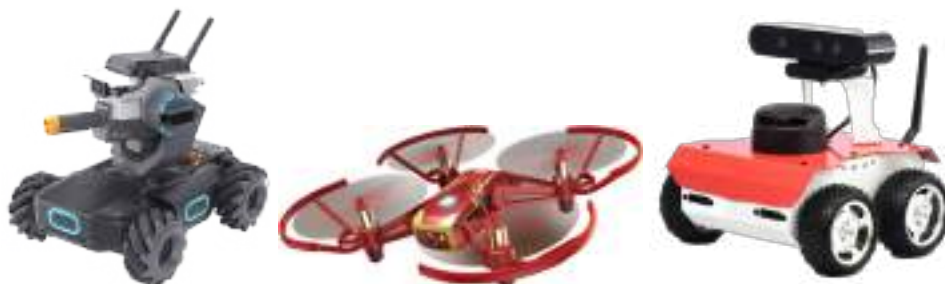
Figure 1. Different AI-enabled educational robots - the DJI RoboMaster S1 robot (left), the DJI Tello Edu drone (middle) and the ROSbot 2 (right), which can be used correspondingly for development, testing and demonstration of algorithms for target tracking, autonomous visual navigation and simultaneous localization and mapping
