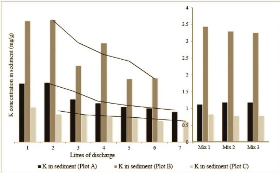
**Fig. 2.** Bar chart showing a decrease in K concentration measured in sediment per litre of discharge for plots A, B and C
