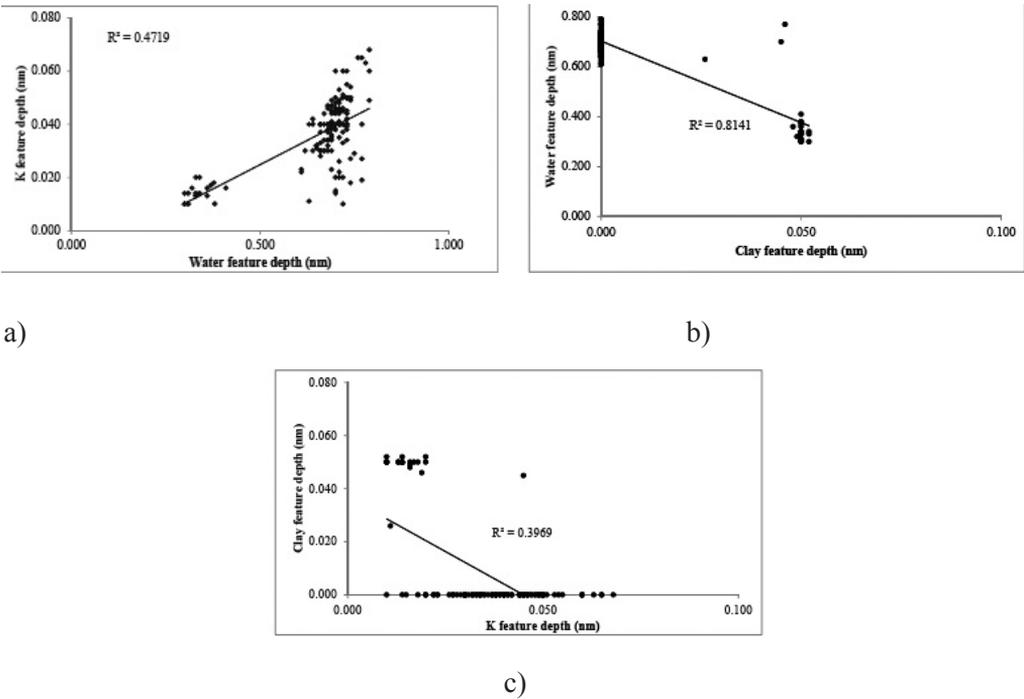
**Fig. 9.** Statistical relationships between depth of water absorption band (1900 nm), clay absorption band (2200 nm) and K absorption band (2465 nm) derived from laboratory spectra measured during a controlled moisture experiment; a) Moisture content vs. K feature depth; b) Moisture content vs Clay feature depth; c) Clay feature depth vs. K feature depth
