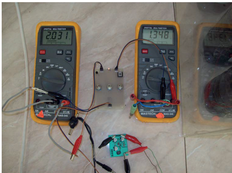
Fig. 5. Experimental set-up of two sensors and a LED powered by LTC3105-PMS connected to nine SMFCs
