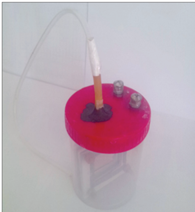
Fig. 1. Photograph of a single-chamber membrane-free MEC reactor
