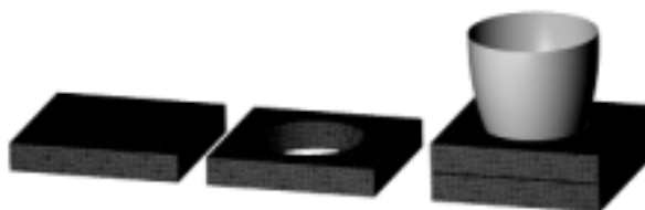
Fig. 1. Plain and holed slabs of silicon carbide and set of slabs (plain at bottom, then one with a hole and china clay crucible placed in hole at top (left to right))
