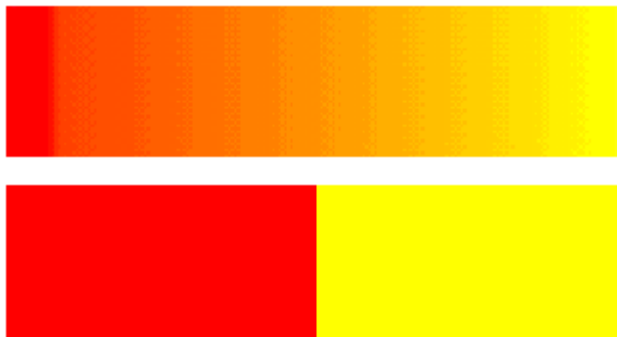
Figure 1. Thermochromism — a schematic presentation: continuous (upper) and discontinuous (lower part). One has to assume that temperature changes continuously when going from left to right.
